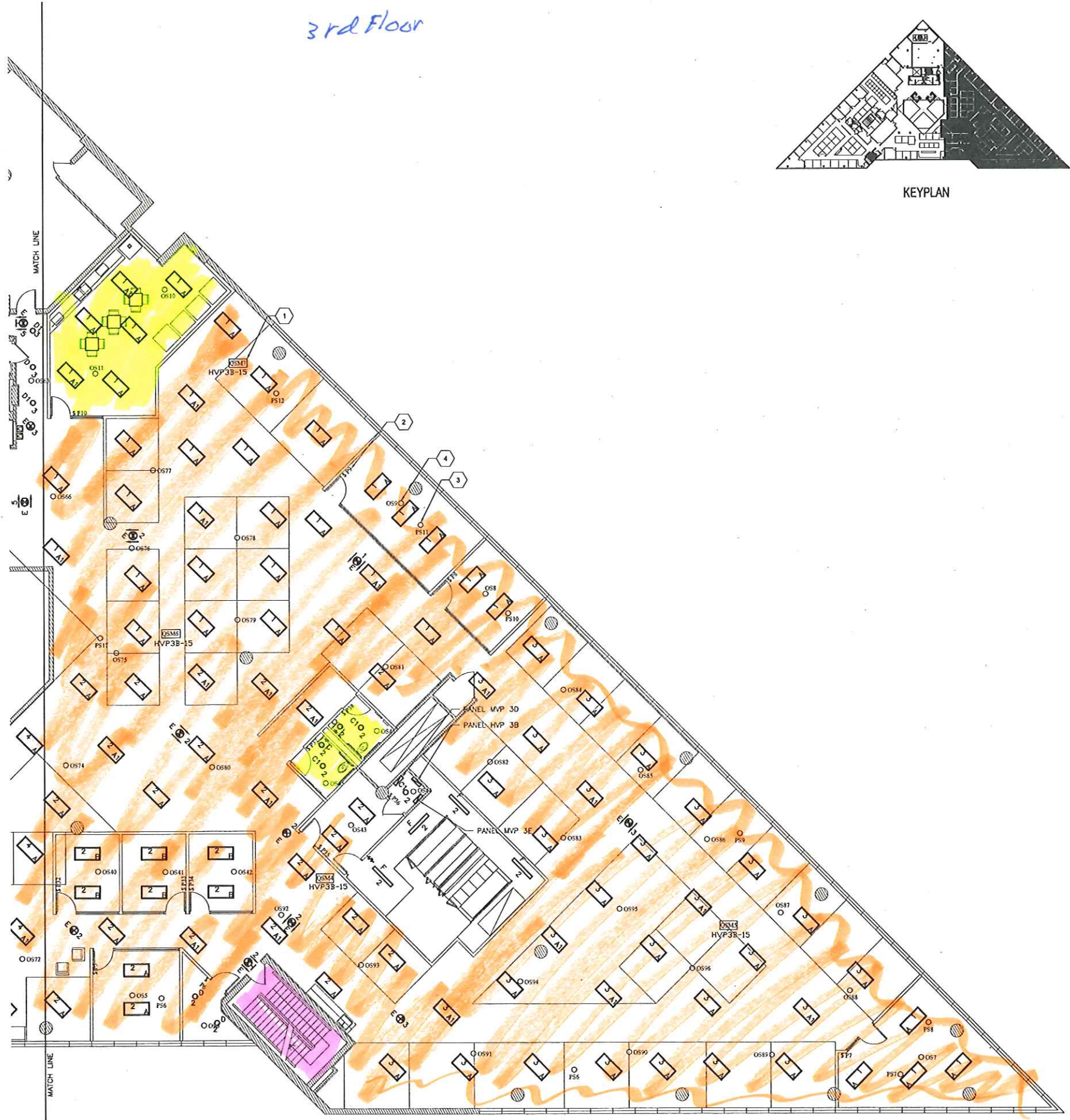
1 THIRD FLOOR EAST LIGHTING PLAN SCALE: 1/8" = 1'-0"
